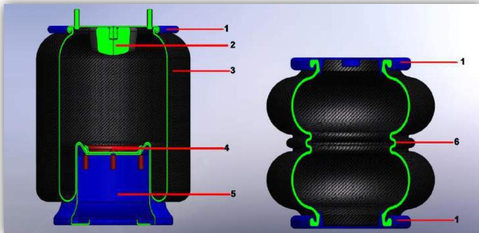
1. The crimped plate serves to fasten the air-spring bellow to the vehicle's frame.
